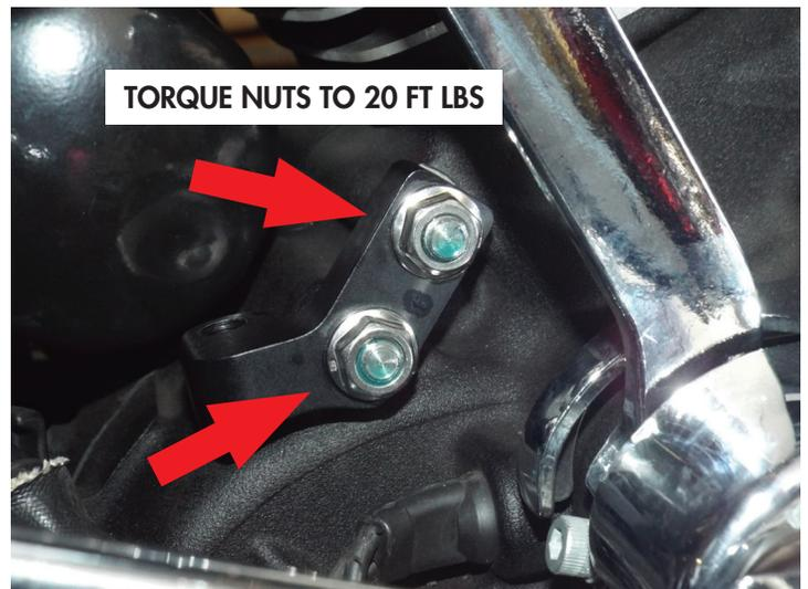
**STEP FIVE:** Install the frame bracket using the 1 ½ long 3/8 bolt with washers – one on the outside of the bracket and two on the inside. (Washer configuration as prior to disassembly.) Use blue loc-tite on all threads, **DO NOT TIGHTEN AT THIS TIME.**
