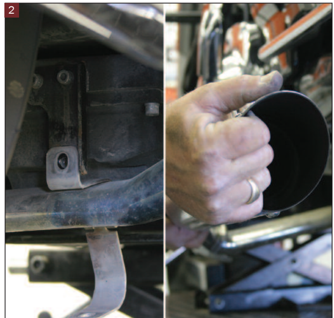
2 The center mounted support strap simply swings out of the way to allow the exhaust pipe and muffler to come off as a single piece.
