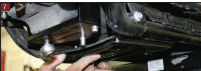
Thread the stainless steel bolts into the oil pan holes.
