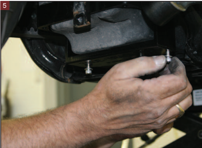
Thread the stainless steel bolts into the oil pan holes.
