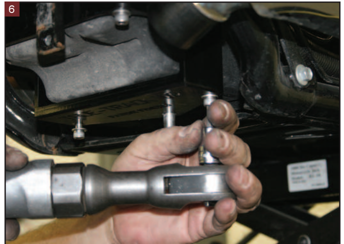
Tighten the bolts completely at this time using a cross pattern so everything gets tightened equally.
