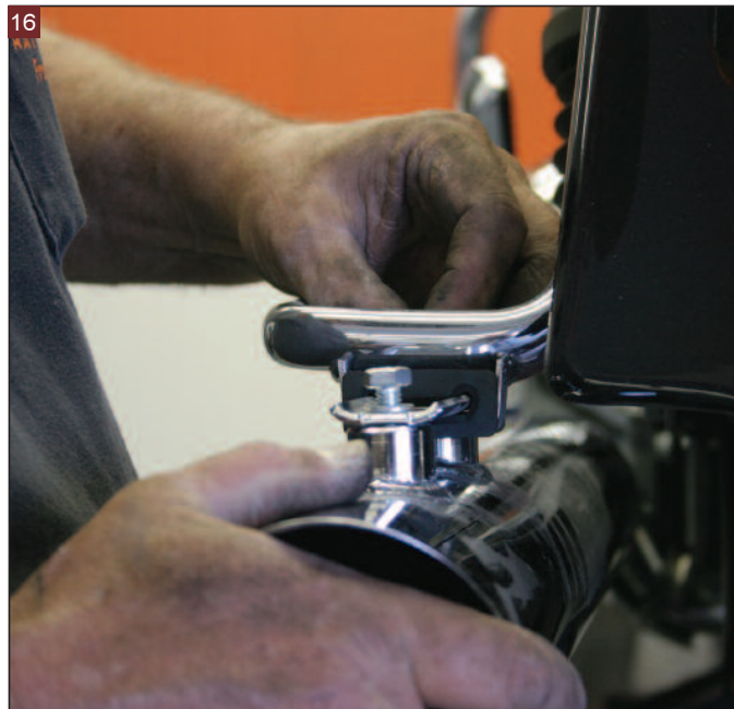
Install the slip-on muffler hardware and tighten it.
