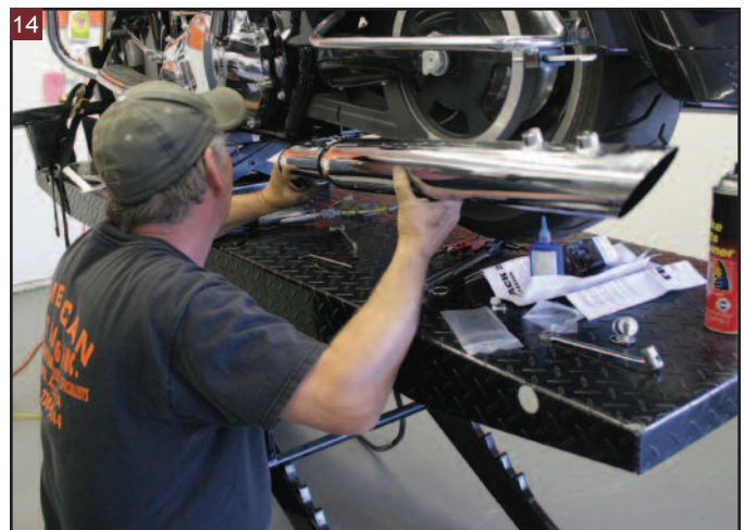
Slip the left side muffler and head pipe back into place on the right side pipe spigot.
