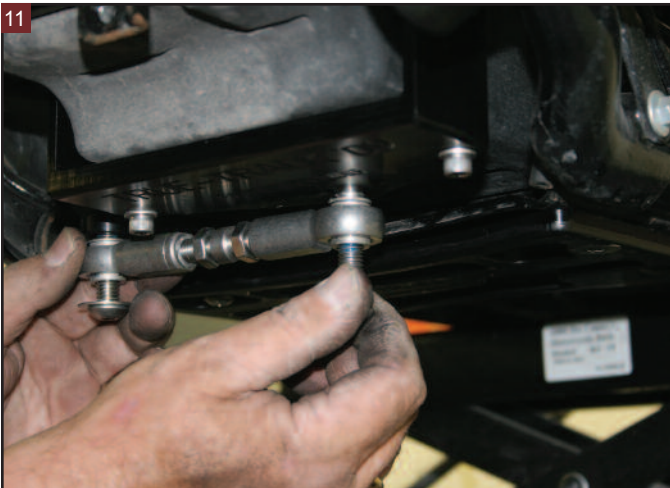
Mount the heim joint on the pins and insert the two bolts into each end.
