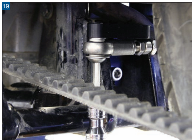
19 Tighten the stabilizing link mounting bolt on the T-bracket.
