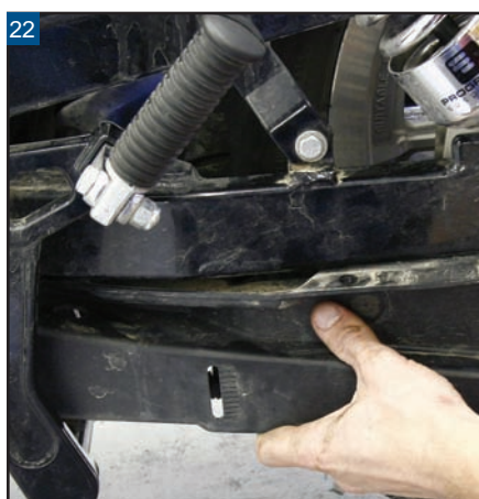
22 Next, slide the lower belt guard back into place.
