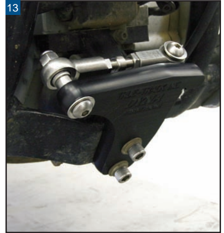
13 This is what the True-Track looks like installed on the front mount of our Dyna Glide.
