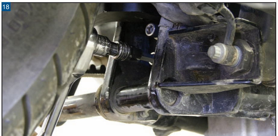
18 Remove the bottom rear motor mount frame bolt and switch it out with one of the provided stainless socket caps. After removing the top bolt, install the T-bracket and stainless socket cap and tighten the mounting hardware.
