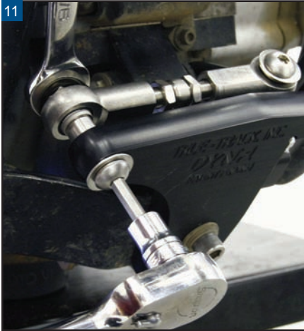
11 Tighten the stabilizer link mounting bolt onto the frame bracket.
