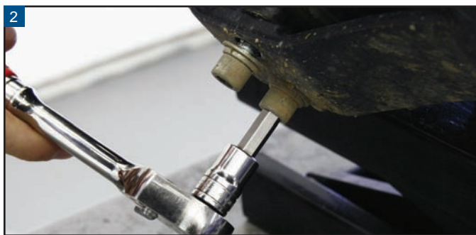
2 Loosen and remove both front mounting screws.
