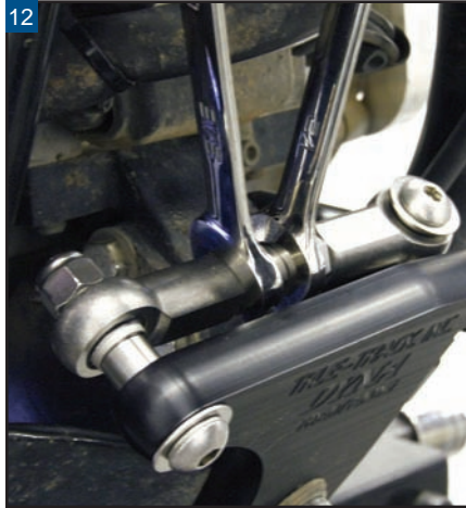
12 While holding the stabilizer link in place, adjust both jam nuts to the outsides of the stabilizer link.
