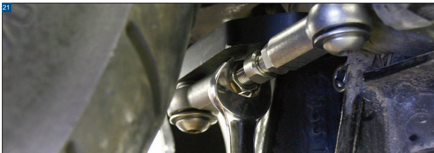
21 While holding the stabilizer link in place, adjust both jam nuts to the outsides of the stabilizer link.
