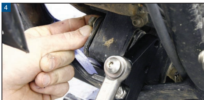
4 While holding the True-Track powertrain bracket in place, start both factory bolts into the threads.
