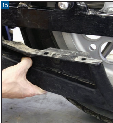
15 With the mounting hardware out of the way, remove the belt guard.
