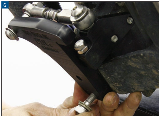
Position the front True-Track frame bracket and start the provided stainless steel bolts. The stabilizer link may have to be adjusted to align the mounting bolts.
