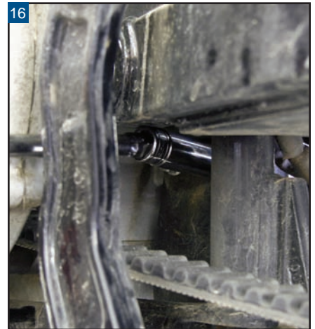
16 Remove the nuts of the rear motor mount using a 9/16" deep socket and a 9/16" box-end wrench.
