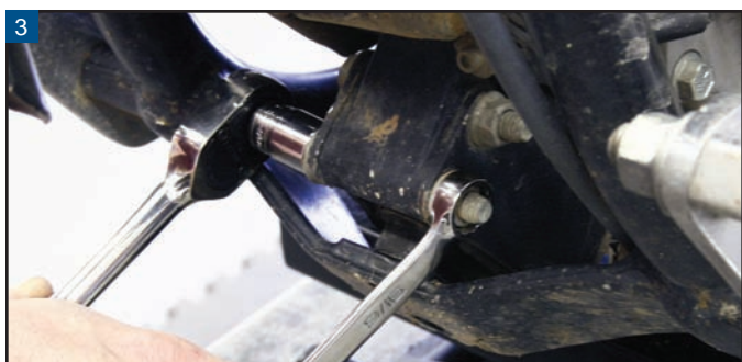
3 Remove the nuts from both front rubber mounting bolts.
