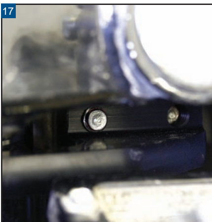
17 Flip the bolts so they come in from the primary side; install the bracket on the brake side and tighten.
