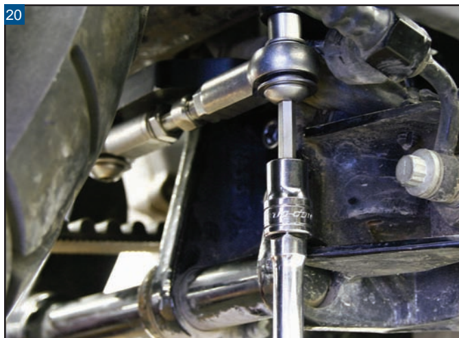
20 Next, tighten the stabilizing link mounting bolt on the powertrain bracket.
