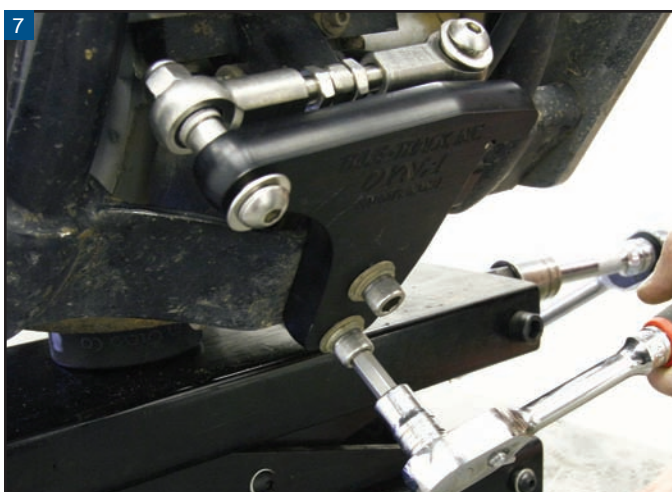
Once in place, tighten both stainless steel bolts.
