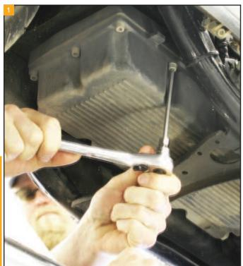
Loosen and remove the bolts holding the oil pan in place.
