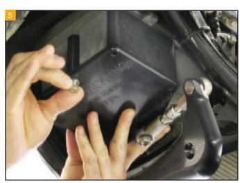
Then, install the True-Track hardware to hold it in place.
