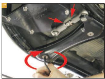
If link is binding, adjust link to a neutral position before continuing.
