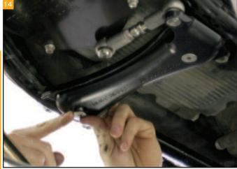
Fit the link in place and install the hardware. Install the dogbone hardware to hold it in place.
