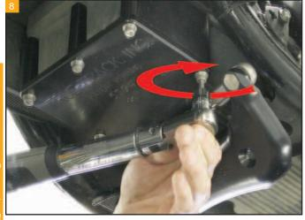
Using a quality torque wrench, torque the pan bolts only after complete assembly.
