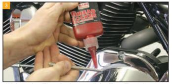
We're using Theadlocker on all the True-Track hardware for a secure lock. True-Track advises Blue Loctite on all hardware threads.
