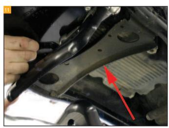
Make sure to check that the cross member is not bent excessively prior to installation of the True-Track.
