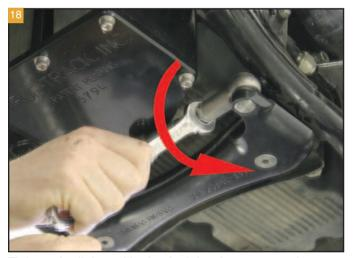
Tighten the link positioning lock hardware securely.
