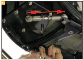
Position the dogbone into place and adjust the link for a proper fit. (Link detached for photo purposes only.)
