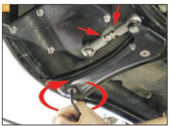
Make sure that the link isn't in a bind as you tighten the dogbone hardware.
