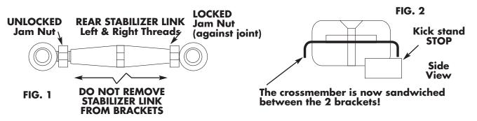
**HOW DOES TRUE-TRACK™ WORK?** It's the third, missing link that is installed at the rear of the power train unit, just like the front stabilizer link and the top stabilizer link combine to keep the power train unit **anchored** in the lateral plane of the frame. The power train unit can **only** move up and down the way it was designed to do.
