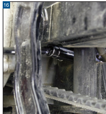
Remove the nuts of the rear motor mount using a 9/16" deep socket and a 9/16" box-end wrench.
