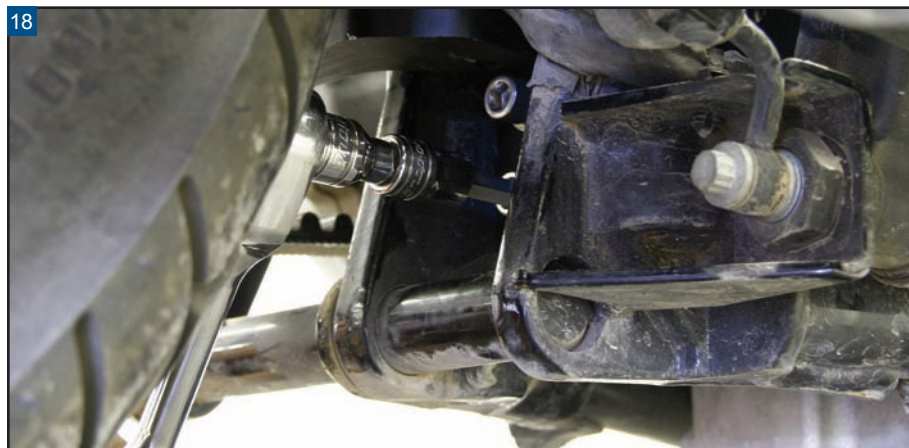
Remove the bottom rear motor mount frame bolt and switch it out with one of the provided stainless socket caps. After removing the top bolt, install the T-bracket and stainless socket cap and tighten the mounting hardware.
