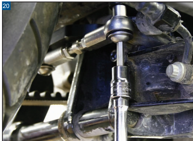
Next, tighten the stabilizing link mounting bolt on the powertrain bracket.
