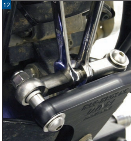
While holding the stabilizer link in place, adjust both jam nuts to the outsides of the stabilizer link.
