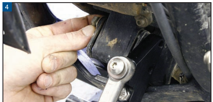
4 While holding the True-Track powertrain bracket in place, start both factory bolts into the threads.
