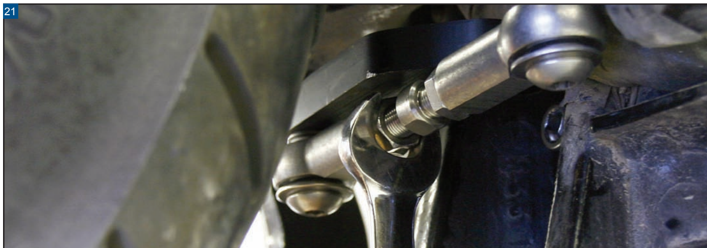
While holding the stabilizer link in place, adjust both jam nuts to the outsides of the stabilizer link.
