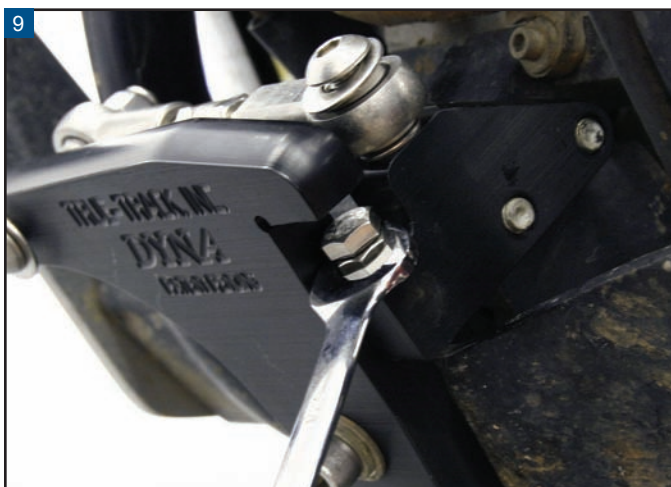
Locking the stop-bolt in place is as easy as tightening the jam nut against the powertrain bracket.
