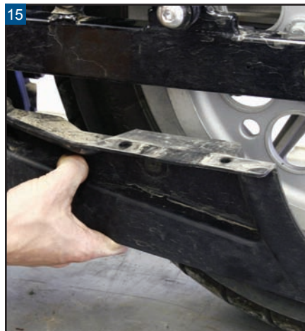
With the mounting hardware out of the way, remove the belt guard.
