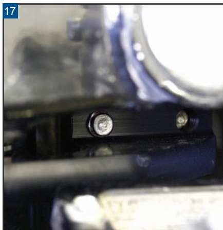
Flip the bolts so they come in from the primary side; install the bracket on the brake side and tighten.
