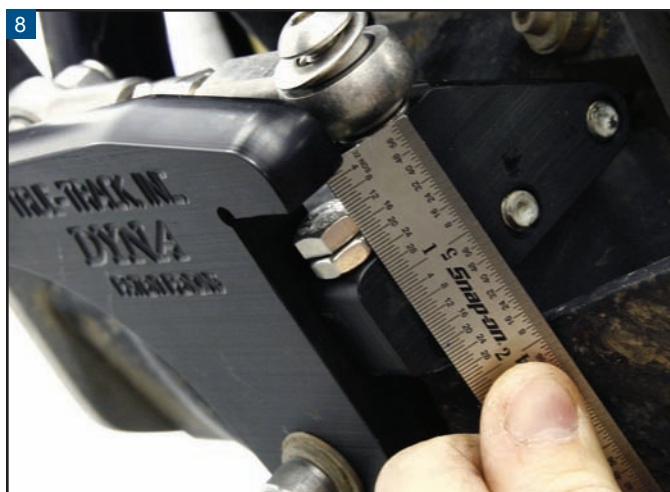
Adjust the stop-bolt on the powertrain bracket to measure 3/8" between the bolt head and the frame bracket.
