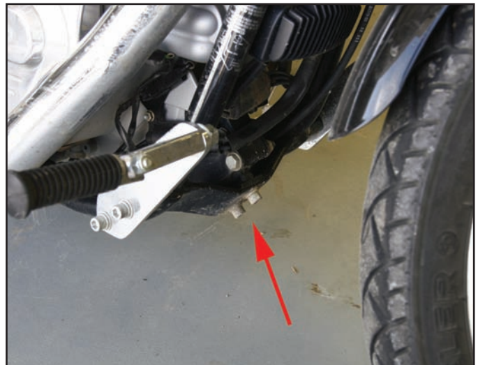
This is the front motor mount area where the front True-Track will mount.
