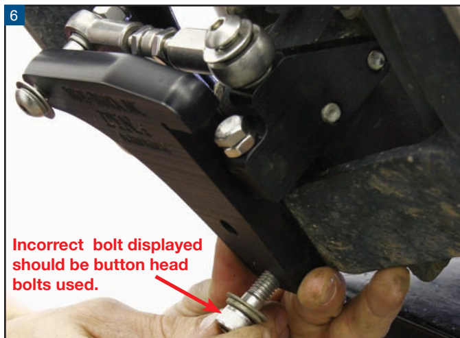
Position the front True-Track frame bracket and start the provided stainless steel button head bolts. The stabilizer link may have to be adjusted to align the mounting bolts.
