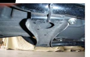
**5** The bucket will mount to the back of the transmission. So we removed the five stock mounting bolts from the back of the transmission pan.
