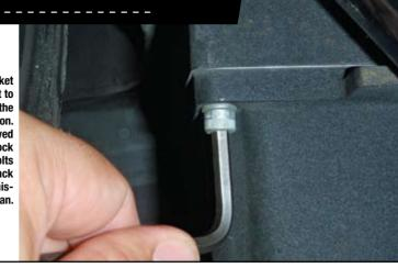
Before installing the True-Track unit, we had to make sure the frame cross member was straight. Sometimes the cross member can get bent from being used as a lifting point for a jack, scraping on a speed bump, or an unexpected off-road excursion. If your cross member is bent, True-Track offers a tool to help straighten it.
