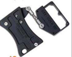
Here is what the True-Track unit for the new '09-present touring models looks like. Installation is essentially the same except it takes a little bit longer on bikes with the crossover pipe running under the bike, as the left-side saddlebag and exhaust have to be removed and reinstalled. Notice the dog bone on this unit is much larger.
