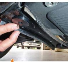
If the cross member is not straight, the pucks won't sit flush and won't line up with the dog bone mounting holes. Our cross member was perfectly straight, so the pucks were dropped into position over the top of the cross brace.
