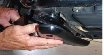
We then lifted the True-track assembly into position and with some thread locker on the bucket bolts that were included, we loosely threaded the bolts into the trans pan and then aligned the dog bone with the cross member and pucks.
