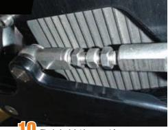
The heim joint is pre-set from True-Track; however, each frame is different and thus some adjustment may be needed, which is why left- and right-hand threads are provided. It is critical that the heim joint be neutral before locking down the jam nuts.
