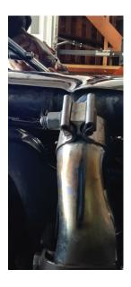
5. Remove the three bolts shown here from the hanger.
