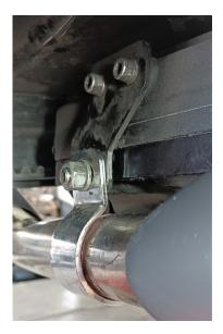
6. Remove the two bolts shown here. Slide exhaust away from cat assembly and lay it to the side.
