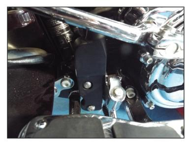
STEP SIX: Install heim joint: attach to both brackets at this time using very little loc-tite
