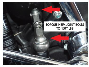
At this time also go back to frame bracket and tighten both bolts to 15 ft lbs
